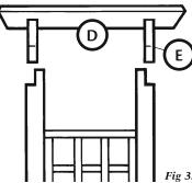
6. Fit the roof assembly onto the posts of the side assemblies and fix at the desired position with screws (x).
