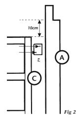
Fit the trellis to the metal brackets using screws (y).
